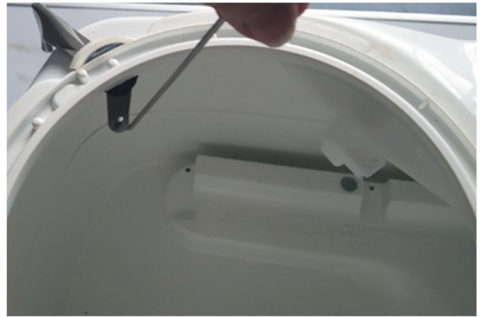
19. Remove the bracket for the locking mechanism from the holders.
