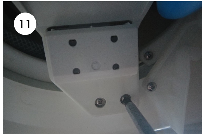
10. Through the service flap, loosen the screws of the the clamps that secure the cables to the base of your Thetford chemical toilet.
