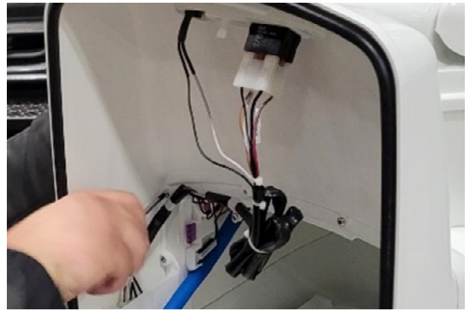
10. Through the service flap, loosen the screws of the the clamps that secure the cables to the base of your Thetford chemical toilet.
