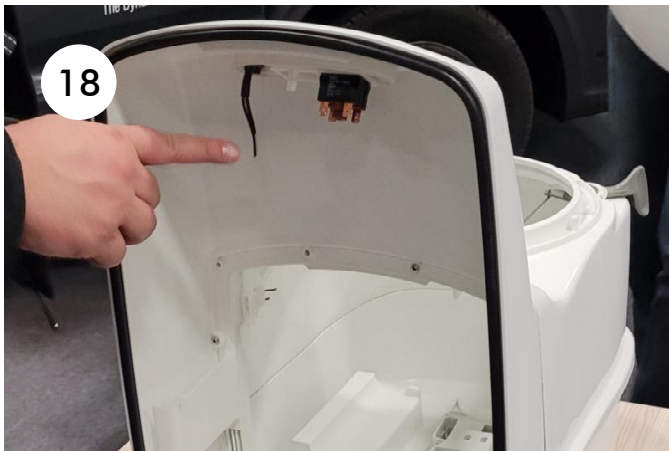
18. Disconnect the cable to the LED or push out the LED.
